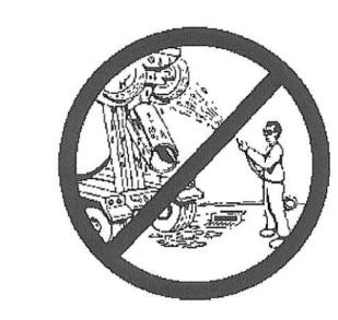
Collect the wash water from washing exposed aggregate concrete and remove it for appropriate disposal off site.
