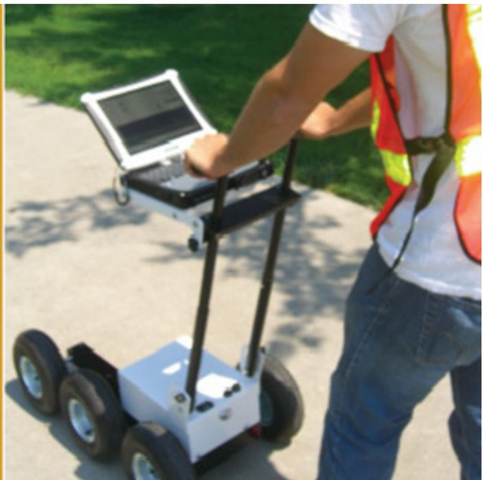
Using Surface Profilers with a Geographical Information System (GIS) is a cost-effective solution to record and map ADA barriers within pedestrian infrastructures.
